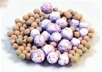
Drysorber colour change, from pale blue to pink, when exposed to water
