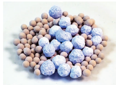
Drysorber colour change, from pale blue to pink, when exposed to water
